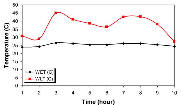
**Fig. 11. Hourly performance of a solar thermal collector panel during the operating hours within a day in January**
