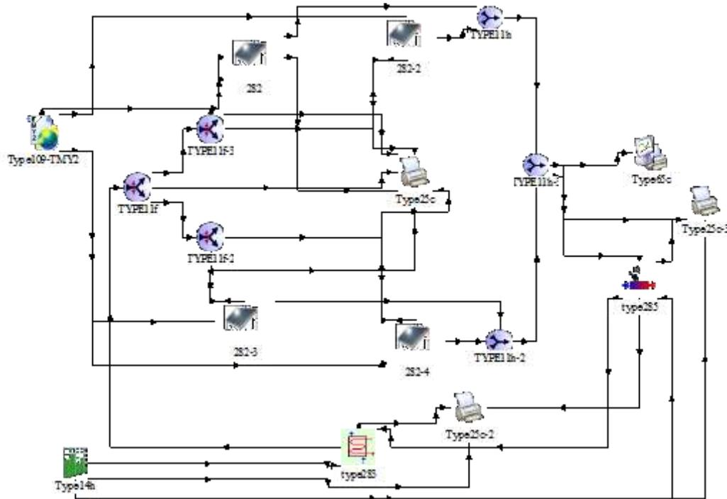
Fig. 6. Simulation layout for a typical array of solar collectors
