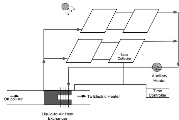
Fig. 5. Schematic diagram for a typical array of solar collectors
