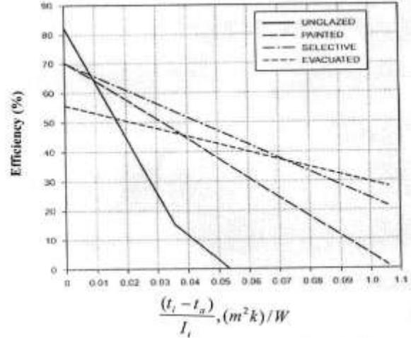
**Fig. 7. Solar collector type efficiencies, [19]**
