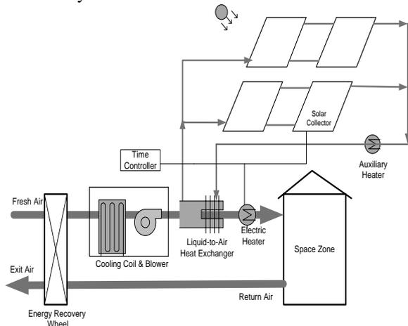
**Fig. 8. Schematic diagram for the HVAC system integrated with the solar collectors**
