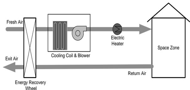
Fig. 2. Schematic diagram for the existing HVAC system
