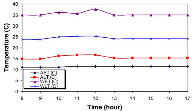
**Fig. 10. Hourly performance of the liquid-to-air heat exchanger during the operating hours within a day in January**
